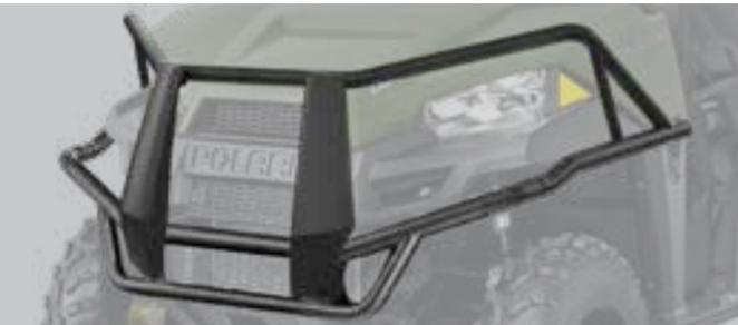
3.2 cm DIAMETER STEEL TUBE CONSTRUCTION
