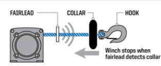
Stops winch at end of pull to prevent driveline stress and plow overlifting
